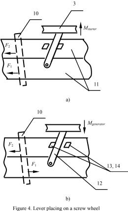
Figure 4. Lever placing on a screw whee 12. lever; 13, 14. support
