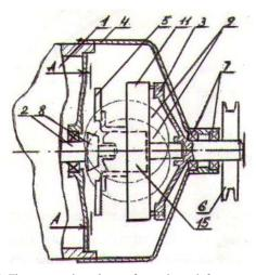
Figure 2. The constructive scheme of actuating unit for starter-generator 1. direct current engine; 2. leading shaft; 3. conducted shaft; 4. cover;
