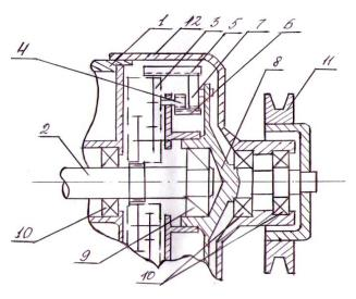
Figure 5. The constructive scheme starting the switching devices 1. direct current car; 2. shaft of the car of a direct current; 3. block of tooth gearings; 4. exit of the block of tooth gearings; 5. rotating the external cogwheel; 6. rotating internal cogwheel; 7. leading cogwheel; 8. pulley shaft; 9. freewheeling muff; 10. bearings; 11. pulley; 12. cover
