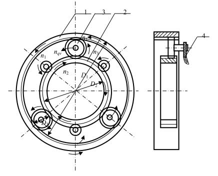
Figure 6. The scheme of placing of external, internal and leading wheels 1. external wheel, 2. internal wheel, 3. driving wheel, 4. pulley shaft
