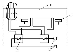
Figure 1. The electric scheme of the generating mode 1. collector; 2. rectifiers; 3. brushes on a rack; 4. contact rings; a and b are the anchor windings
