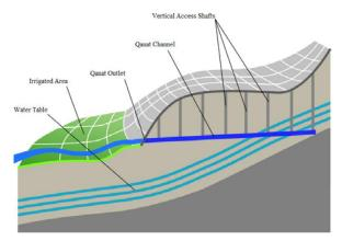
Figure 12. Schematic diagram of Qanat construction [12]
