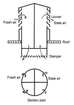
Figure 9. Schematic view of new wind catchers [7].
