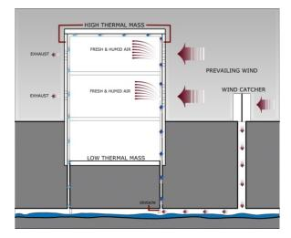
Figure 13. Suggested model for water usage and underground cooling system in desert buildings
