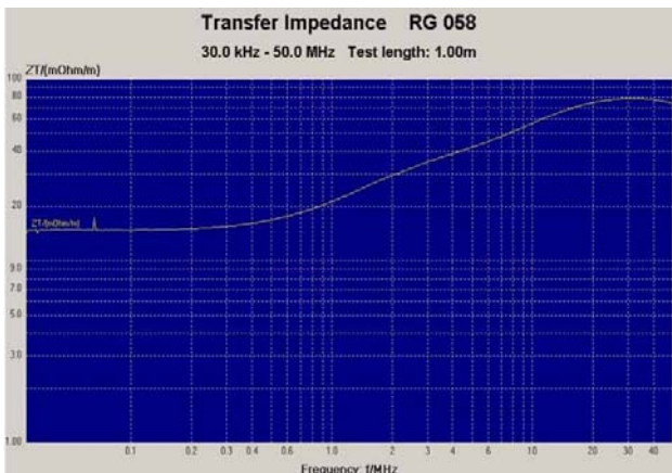
Figure 10. RG-058 cable-Transfer impedance-frequency variation using tri-axial method
