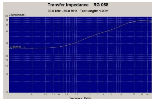
Figure 4. Frequency response of RG 058 antenna cable transfer impedance
