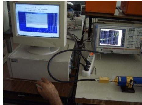
Figure 2. Connecting test setup to circuit analyzer with WinComet program
