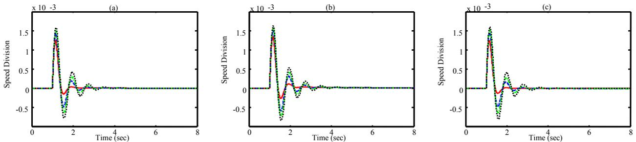
Figure 5.  $\Delta T_m=0.1$  (p.u.) under  $X_c=0.6$ ; CPSO (dotted), PSO-TVIW (dashed-dotted) and PSO-TVACPSS (dashed) and GSA (solid) (a)  $P=0.8, Q=0.4$  (b)  $P=0.5, Q=0.1$  (c)  $P=1.0, Q=0.5$
