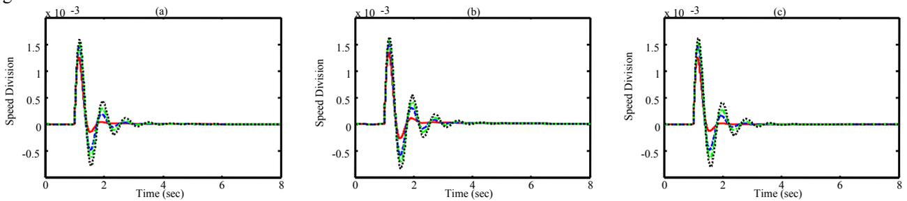
Figure 4.  $\Delta T_m=0.1$  (p.u.) under  $X_c=0.3$ ; CPSO (dotted), PSO-TVIW (dashed-dotted) and PSO-TVACPSS (dashed) and GSA (solid) (a)  $P=0.8, Q=0.4$  (b)  $P=0.5, Q=0.1$  (c)  $P=1.0, Q=0.5$
