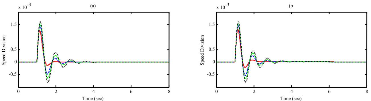
Figure 9.  $\Delta T_m=0.1$  (p.u.) under  $X_c=0.6$  and  $H=H/4$ , CPSO (dotted), PSO-TVIW (dashed-dotted) and PSO-TVACPSS (dashed) and GSA (solid)
