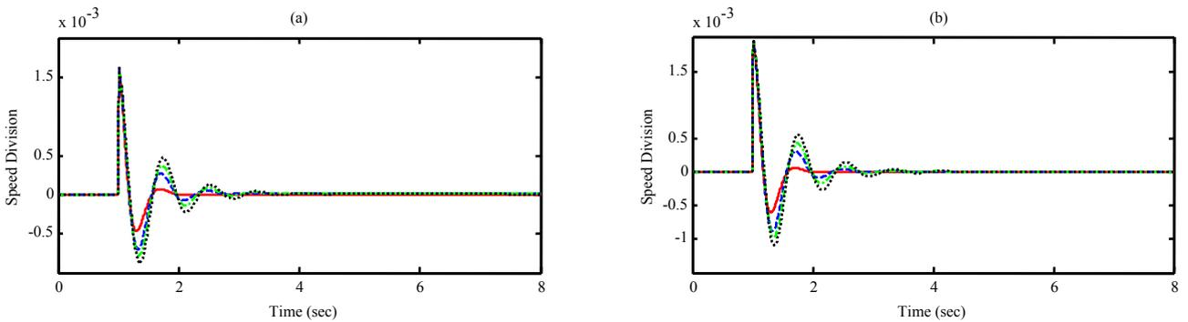
Figure 8. 3-phase to ground fault 100 msec for  $X_c=0.3$ , CPSO (dotted), PSO-TVIW (dashed-dotted) and PSO-TVACPSS (dashed) and GSA (solid)
