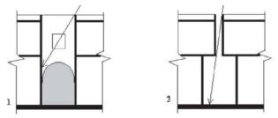
Figure 12. Different structures to provide more shadow in the public streets in hot arid climate
