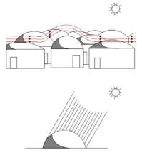
Figure 8. Openings on the dome shaped roofs are ventilation and daylighting elements
