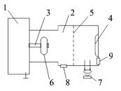
Figure 1. Block scheme of an experimental assembly 1- high voltage nanosecond generator, 2- vacuum chamber, 3- cathode, 4- anode, 5- metal netting, 6- fluoroplastic cap, 7- electron-optical camera, 8- shunt for measuring of discharge total current, 9- shunt for measuring of electron beam's current
