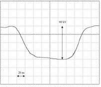
Figure 2. Oscillogram of high voltage pulse
