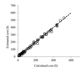
Figure 8. Proposed algorithm accuracy in calculating the load shedding cost considering load priority
