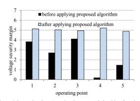
Figure 6. Improving the VSM using the proposed algorithm for selected operating points
