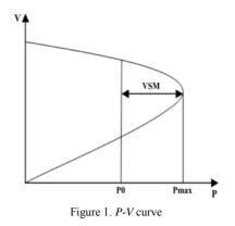
In this study, the authors used an ANN for estimating voltage stability based on the *VSM* index. At the top speed of PMUs, the information of these units can be used to provide the necessary data for the ANN in order to estimate the *VSM*. The *VSM*, then, that is required for safe operation of the network depends on the amount of tension value in the power system.
