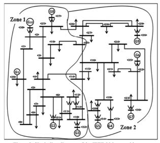
Figure 3. Single-line diagram of the IEEE 39 buses with areas considered
