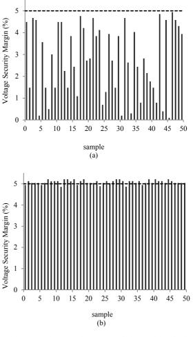
Figure 5. Voltage security margin (a) before applying the algorithm (b) after applying the algorithm
