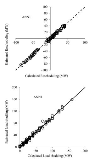
Figure 4. Proposed algorithm accuracy in estimation of generator production pattern changes and load shedding value for ANN1
