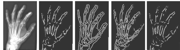
Figure 5. Edge operators: (a) Original image, (b) Prewitt, (c) Canny, (d) Laplacian of Gaussian, (e) Roberts
