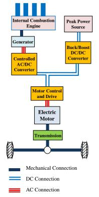
Figure 1. Series connection Hybrid Electric Vehicle
