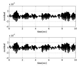
Figure 6. Two residual signal with improper value of  $\gamma = 0.00023$ , the fault occurrence is impossible to detected
