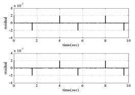
Figure 4. Two residual signal with proper value of  $\gamma = 0.0000023$ , that represent the fault occurrence due to Figure 3
