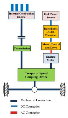
Figure 2. Parallel connection Hybrid Electric Vehicle
