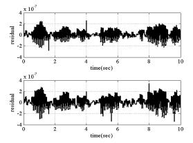
Figure 5. Two residual signal with improper value of  $\gamma = 0.00023$ , the fault occurrence is difficult to detected
