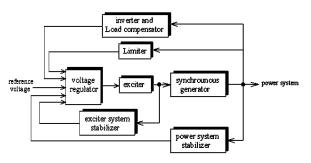
Figure 1. Block diagram of synchronous generator excitation system and structure diagram of power system stabilizer
