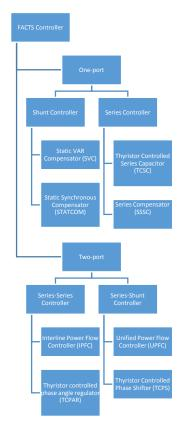
Figure 3. Overview of compensation devices [1]
