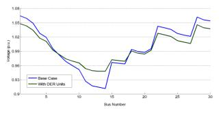
Figure 5. Voltage profile before and after implementation of DER units for the best solution of case 2
