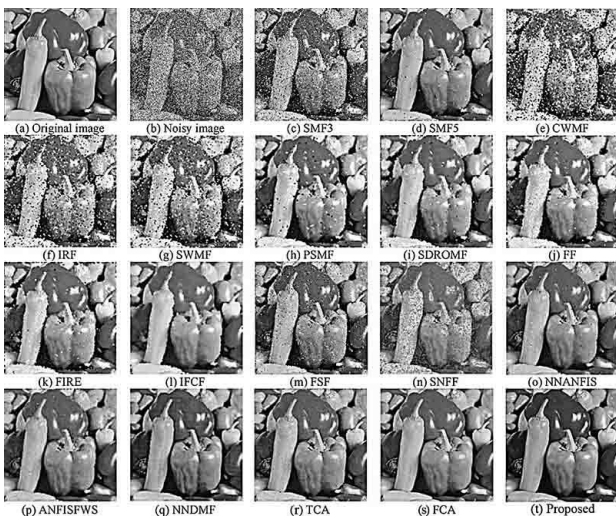
Figure 3. Comparison of the enhanced images for the Peppers by impulse noise density of 50%
