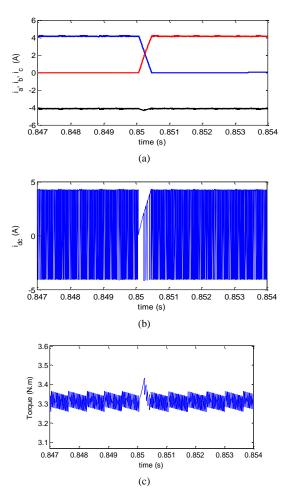
Figure 8. Simulation results in the high speed range (1500 rpm), (a) Phase currents, (b) DC-link current, (c) Commutation torque ripple
