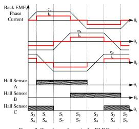
Figure 2. Signal waveforms in the BLDC motor
