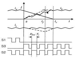
Figure 3. Switching patterns and commutation in low speed [6]
