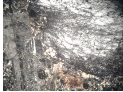
Figure 9. Sino diorite microscopic cross section (XPL, 50x)
