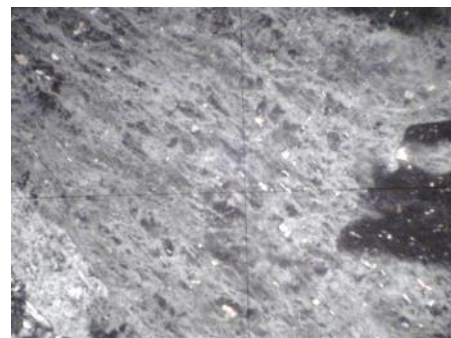
Figure 10. Monzodiorite microscopic cross section (XPL, 50x)
