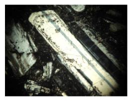
Figure 8. andesite microscopic image (XPL, 50x)
