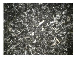
Figure 7. Andesite microscopic image (XPL, 50x) microliter texture in andesite
