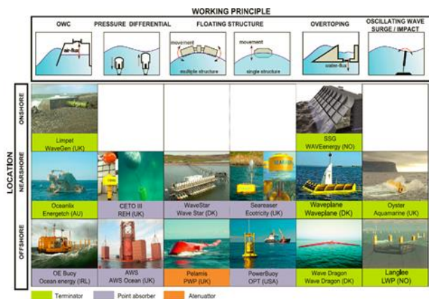
Figure 1. Grouping of systems that produce electrical energy from wave energy [1]
