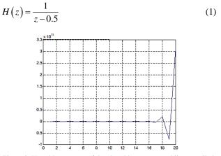
Figure 2. Unstable response of the closed loop system while controlled by a discrete PID controller (excited by a unitary step)
