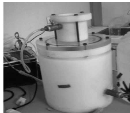
Figure 2. Photograph of Radon diffusion measurement system [16]
