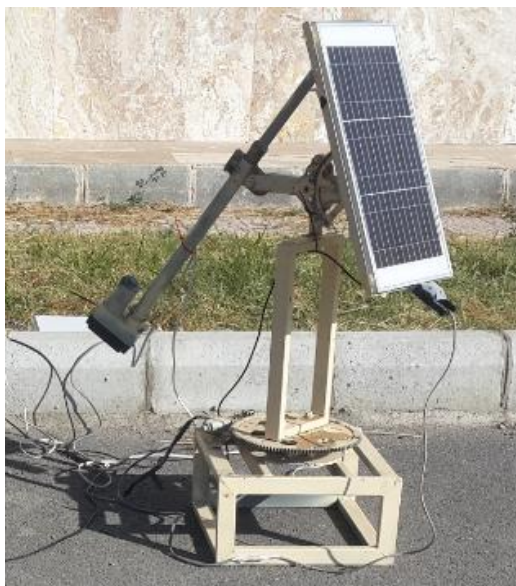
Figure 2. PV system with tracker
