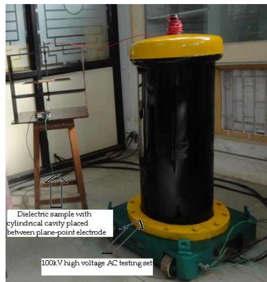
Figure 7. Experimental setup condition with high voltage source
