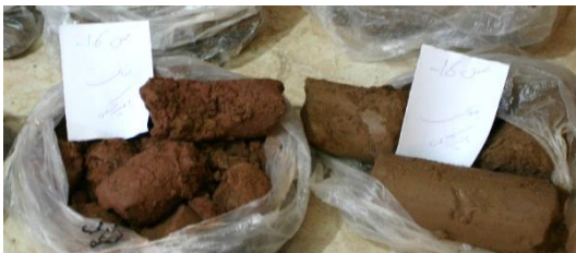
Figure 3. Specimens taken from the drilled boreholes
