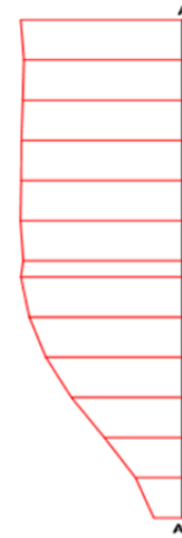
Figure 5. Horizontal deformation of the embankment in behind cover
