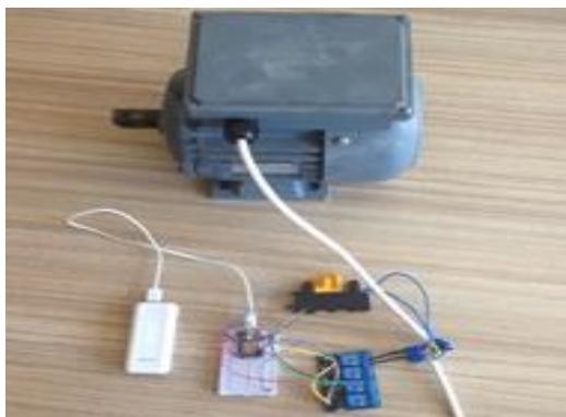
Figure 11. View of the remotely controlled motor
