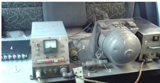
Figure 4. Measuring - recording equipment for testing car, 1- gyroscope CGV-5; 2- transducer of angular accelerations AVS-45 AC; 3- accelerometer MP-95; 4- MtPro-2 measuring complex; 5- central control panel; 6- remote control; 7- power supply
