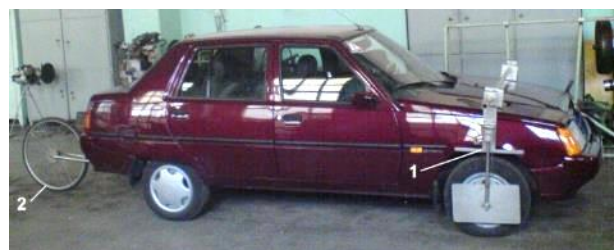
Figure 1. Vehicle with research equipment, 1- measurement device of toe-in angles and turn; 2- "the fifth" wheel of measuring complex
