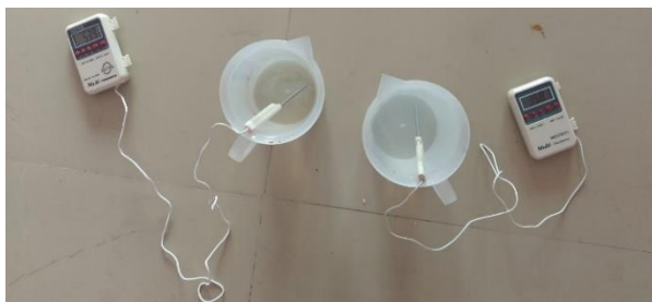
Figure 2. Measurement at outlet through digital thermocouple
