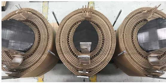
Figure 2. Winding configurations of the three-winding transformer
