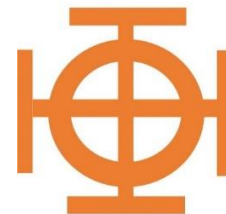
Figure 4. Top view of unit cell of inkjet printed MA [57]
