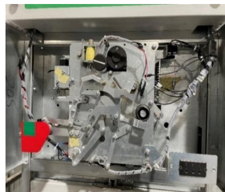
Figure 9. Motorized mechanism tested for mechanical endurance
