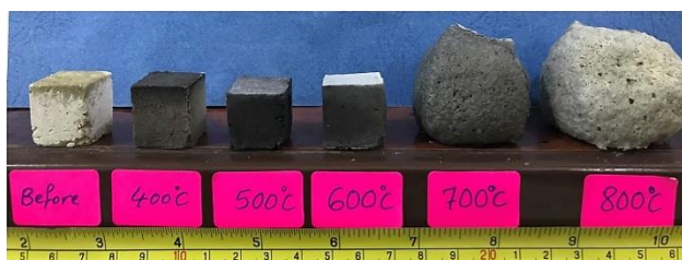
Figure 6. MGY2-N8 specimen's mages before and after thermally curing between 400-800 °C / 1 hour
