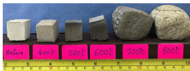
Figure 3. MGY0.5-N8 specimen's mages before and after thermally curing between 400\text{-}800 \text{ }^\circ\text{C} / 1 \text{ hour}
