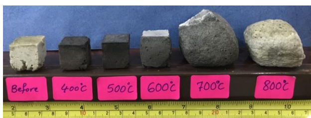
Figure 5. MGY1.5-N8 specimen's mages before and after thermally curing between 400-800 °C / 1 hour
