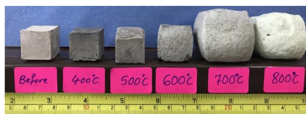
Figure 2. MG-N8 specimen's images before and after thermally curing between 400\text{-}800 \text{ }^\circ\text{C} / 1 \text{ hour}
