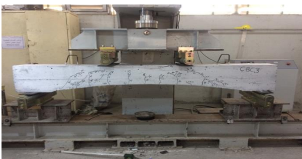
Figure 33. Cracks in CBC3 beam
