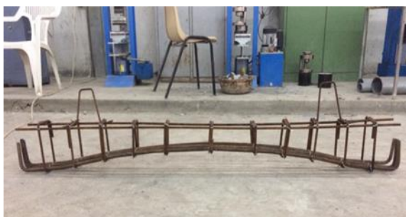
Figure 11. Details of reinforcement for CBC3
