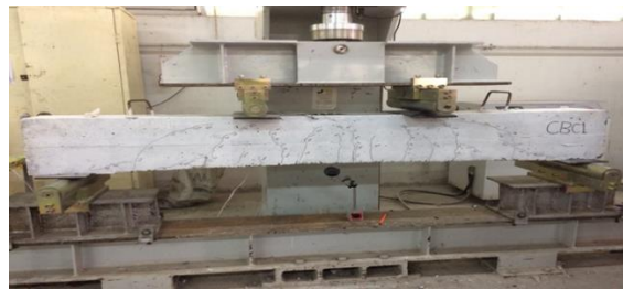
Figure 31. Cracks in CBC1 beam
