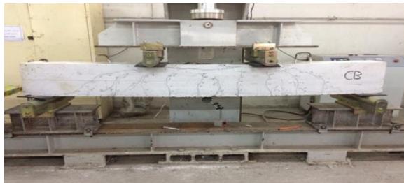
Figure 30. Cracks in CB beam
