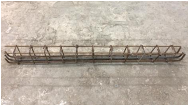
Figure 8. Details of reinforcement for CB specimen
