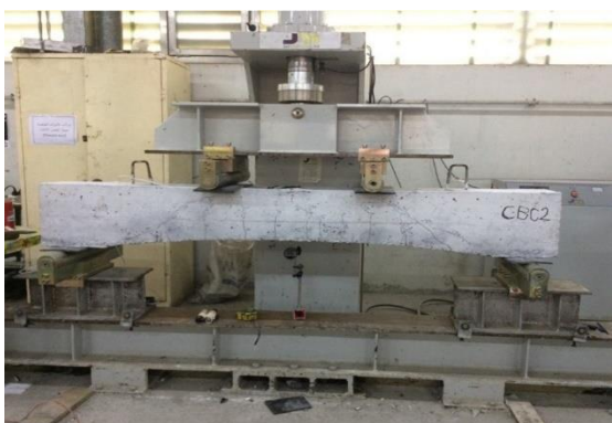
Figure 15. Test setup of CBC2
