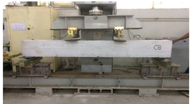
Figure 13. Test setup of CB
