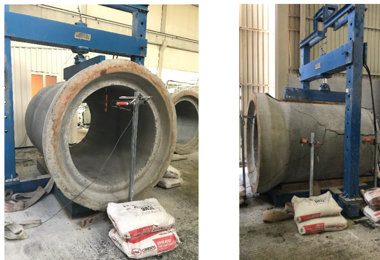
Figure 6. Testing of the fiber concrete pipe [2]
