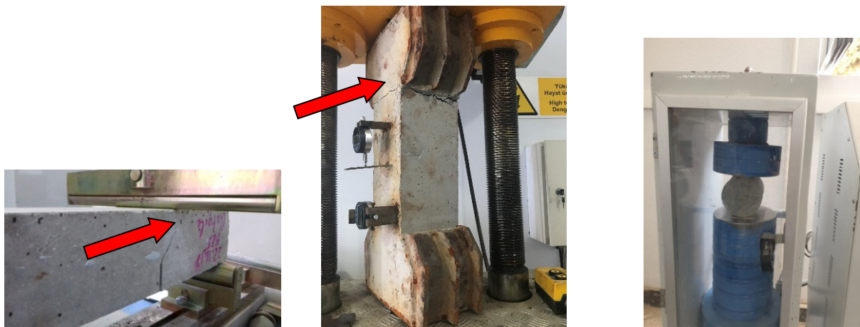
Figure 5. Testing of the fiber concrete samples [2]
