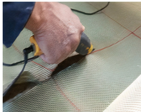
Figure 1. Cutting carbon/Kevlar fibers with EC [25]
