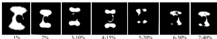
Figure 4. Small-angle radiographs of LDPE oriented at room temperature (1) then free-shrunk at T=100\text{ }^\circ\text{C} (2), re-stretched at room temperature (3)-(7) [5, 6, 8]
